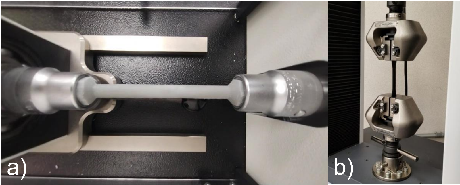
Figure 2 a) Torsion test fixture, b) tensile test fixture
