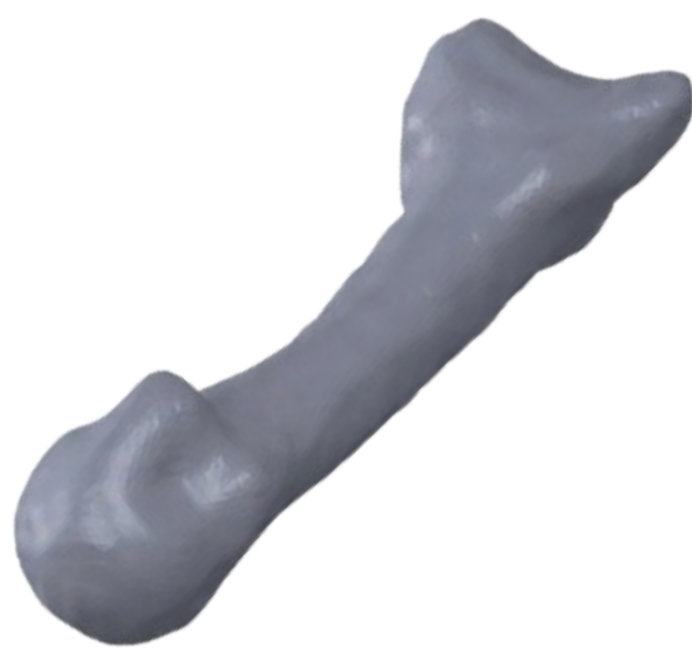
Figure 1. Initial morphological model of a human metacarpal, utilized as the design domain for structural synthesis.
