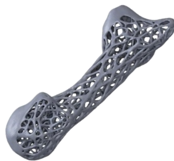
Figure 2. Topologically optimized projection exhibiting a bio-inspired lattice with hierarchical porosity to maximize the stiffness-to-weight ratio.
