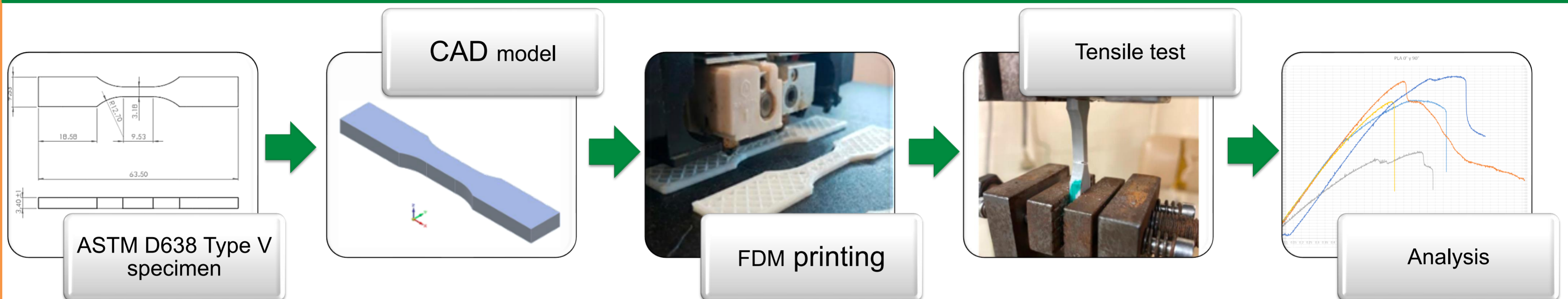
Fig. 1 Experimental procedure for PLA tensile testing.
